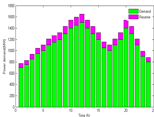
Figure 2 Power demand and reserve for 10-unit test system
